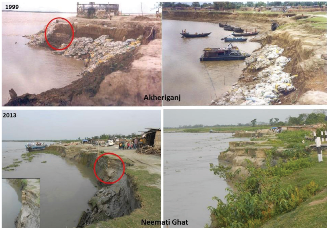
Figure 10. Riverbank failure due to presence of sandwiched sand layer (marked by circle) — highly vulnerable zone along the Ganga, at Akheriganj, West Bengal (upper panel); the Brahmaputra at Neemati Ghat, Jorhat, Assam (lower panel).
