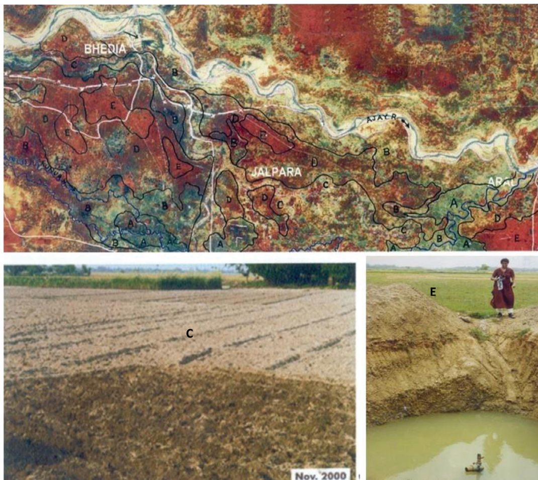
Figure 9. Geo-environmental mapping during flood situation, 2000, for locale-specific flood management (Bhedia-Jalpara-Aral), along the Ajay River. A = Deep and long-lasting inundation; B = Deeply Submerged; C = Submerged but drains off well; D = Shallowly submerged; E = Rarely submerged (Base of the image: 27.9 km; Central coordinates: 23°39'12" N, 87°45'54" E).
