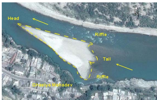
Figure 5. Longitudinal bar near Ghasiya Mahadev (Google Earth Image, 2013)
